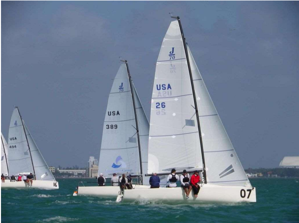
Sail No. 26 is a great example of pulling on the cunningham and seeing the first 10% of the sail go smooth, indicating the wrinkles are in fact from overbend. Courtesy Steve Hunt
