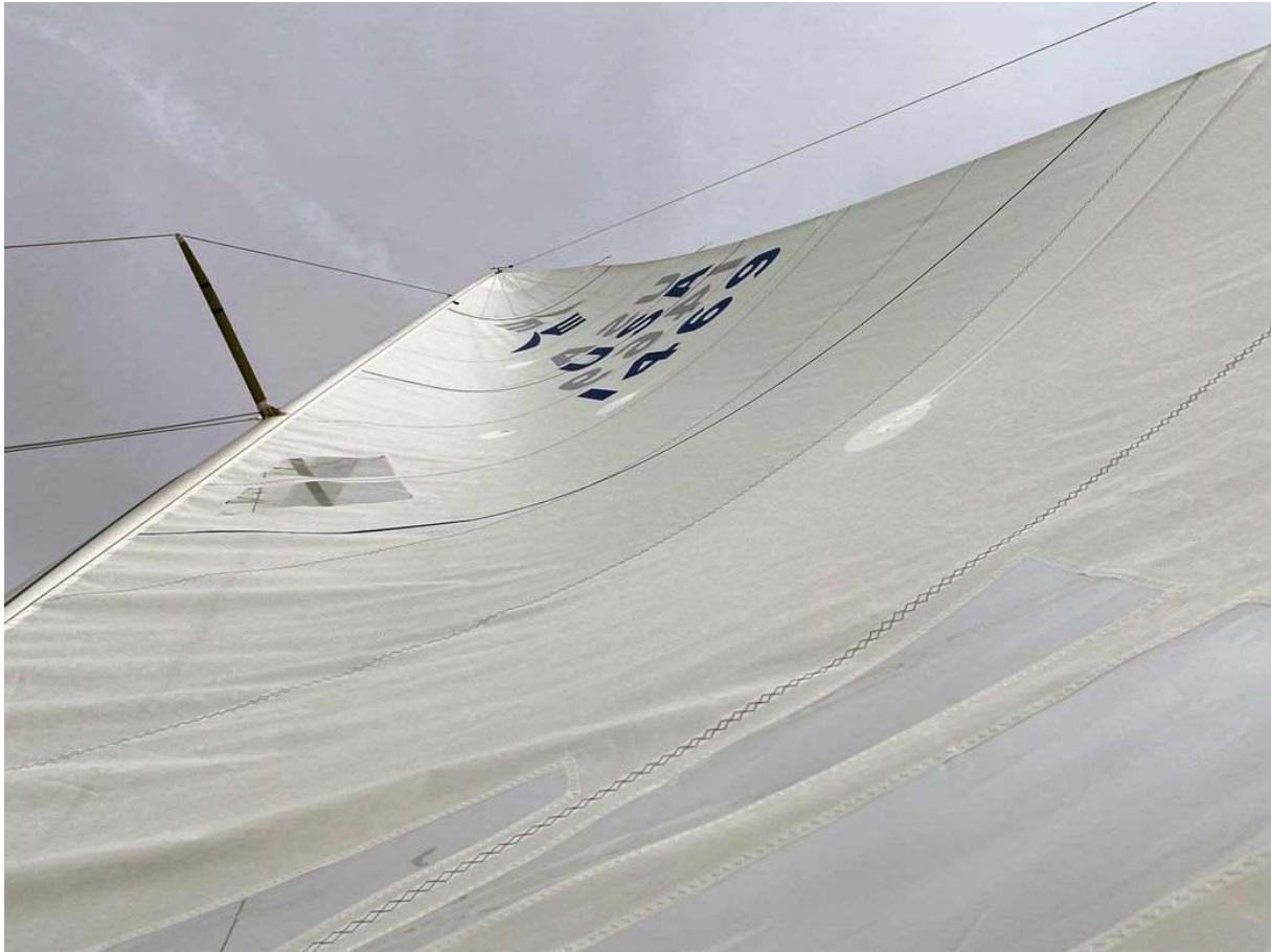
Contraction wrinkles usually happen down low and tend to run almost parallel to the boom. Courtesy Steve Hunt
